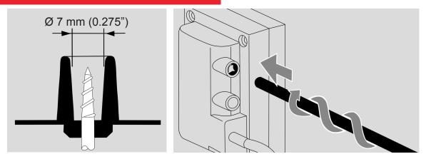
These transformer models use a spearlock connection and accept 7 mm ignition cable. Install the ignition cable by "twisting" or "screwing" it into the spearlock connection, which resembles the business end of a screw. Once installed, tug on the ignition cable firmly to ensure an adequate connection. Use of excessive force is not necessary, and may damage the equipment.
